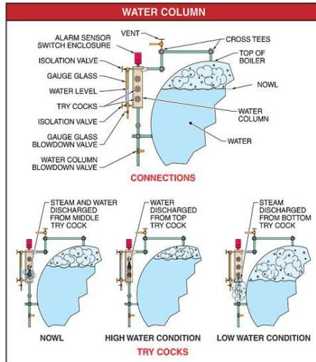
All steam boilers must have two methods of determining the water level in the boiler. The gauge glass is the first and easiest method for determining boiler water level. A second method for determining boiler water level is try cocks. *Try cocks* are valves located on the water column used to determine the boiler water level if the gauge glass is not functional.
