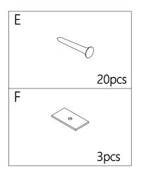
Place the items front face on a protective surface as per image. Align the backing part 9 and 10 install part E fixings to all 5 corners once aligned install all remaining fixings.
